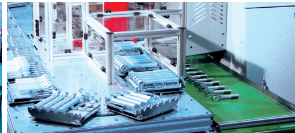
20-station pallet magazine with customer-specific pallets
