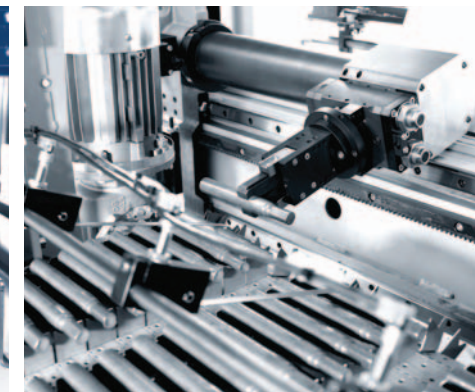
Chain feeding system with V-supports for preformed shaft parts of various shapes.
