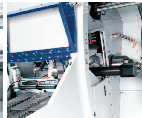
Fully automatic shaft loading. Feed-in via a conveyor belt, removal via the finished parts pick-up device.
