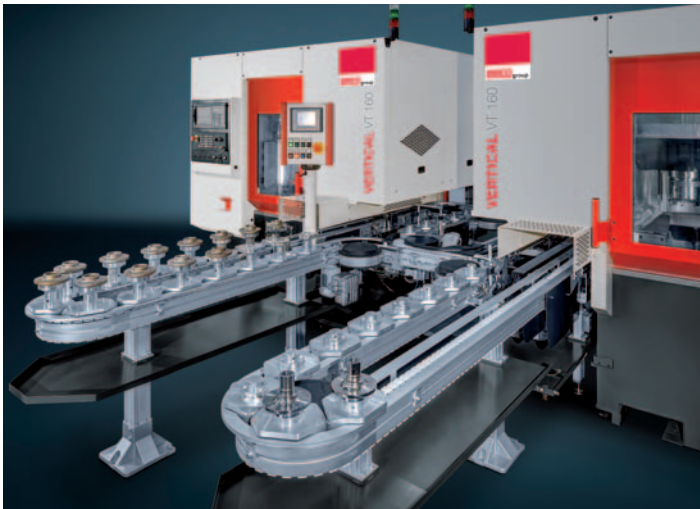
The DUO VT is available as a meander design, which is equipped with a 180° turner and an optional switch. Up to 25 pallets can be used per operation. Separate controls exist for different operating modes (manual, setup, automatic).
