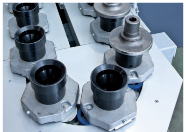
The machines can be equipped with different conveyer belts. One possibility is the standard linking system from pallet belts with spring-operated pick up stations, including 20 workpiece carriers. The feed direction is clockwise. The belt is placed completely under the machines.
