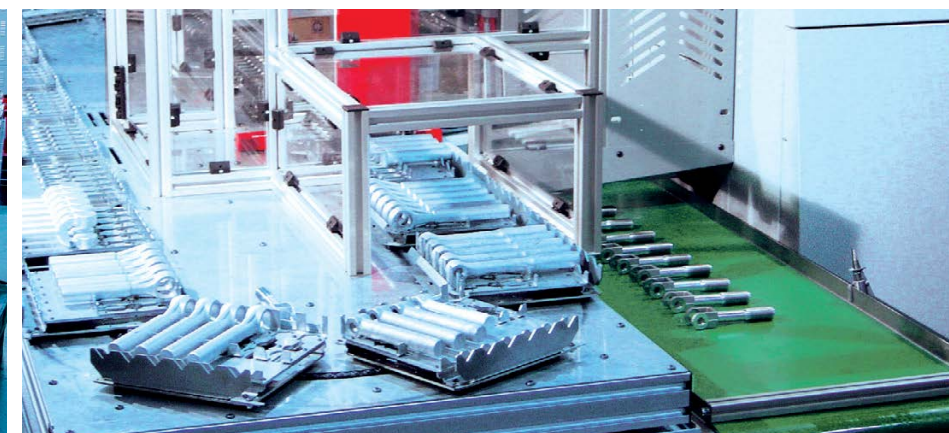
20-station pallet magazine with customer-specific pallets
